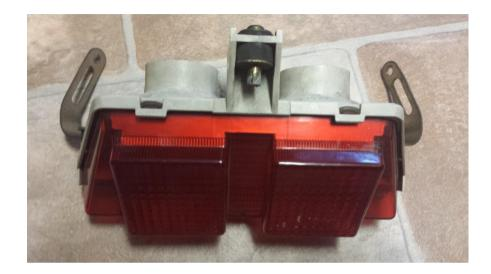
The red lens is glued in place. The glue softens when hot, and the best method is to soak it in hot water from the tap, mixed with some from a boiled kettle. Soak for a good 5 minutes so the heat gets in (gets a good clean too).
