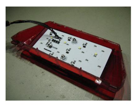
Heat the back reflector back up so the glue softens, and then push the lens back into place.
