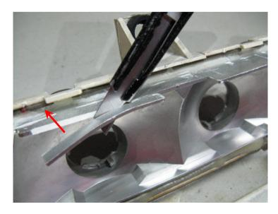
Sit the module in the lens and mark the two hole locations on the lens.
