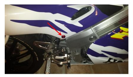
With the fairing removed, you will be able to unscrew the brakelight.
