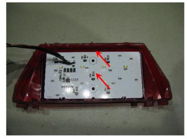
Drill both holes with a 4mm drill. Drill very slowy. Brittle plastics will chip and crack around the edge if you drill through too quickly. Go slow for the win.
