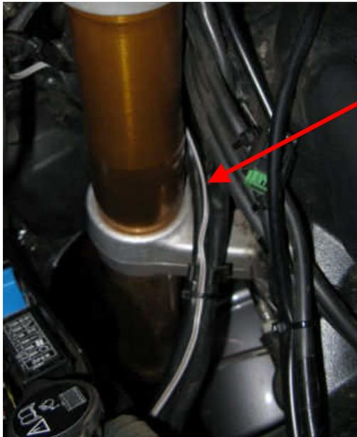
Route the daylight sensor wire along the same path as the other wire harness. So it spirals around the suspension fork.
