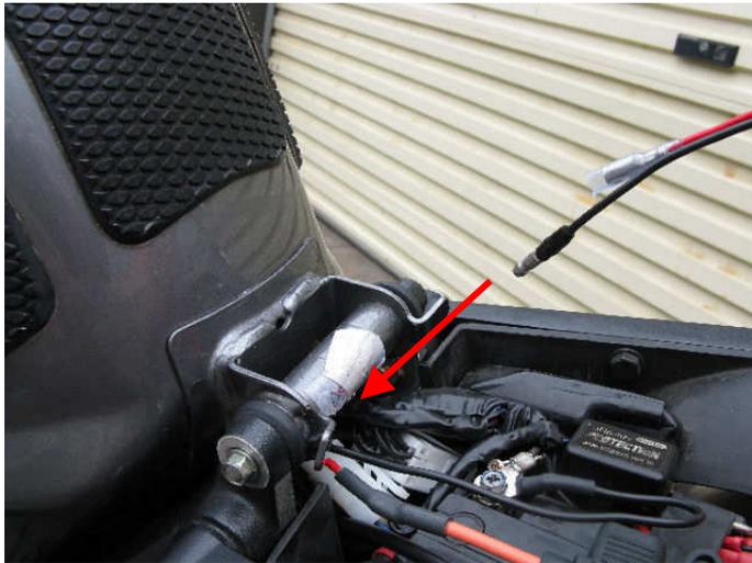
Feed the battery cable under the rear tank hinge.
