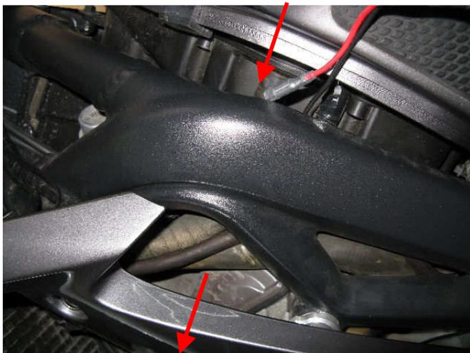
Feed the cables behind the frame and behind the cables.
