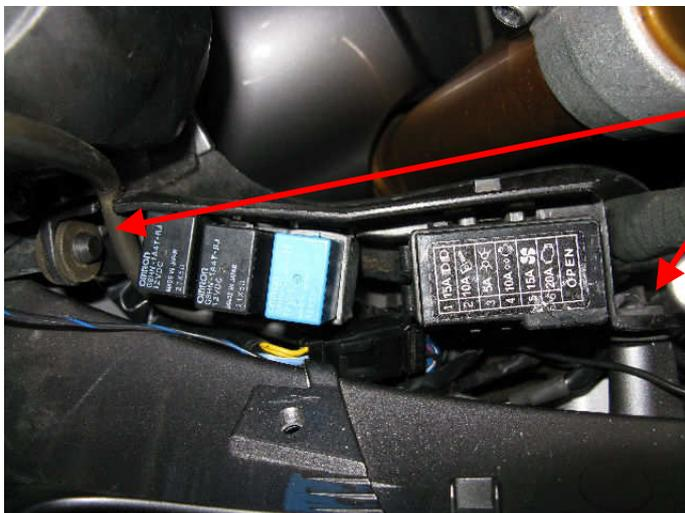
To get to the headlight connector, move the fuse/relay bracket off it's pegs.
