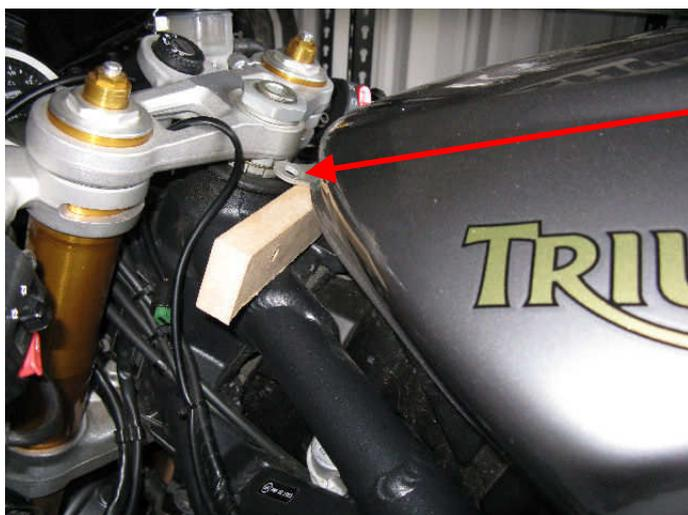
Remove the 2 bolts holding the front of the tank.
