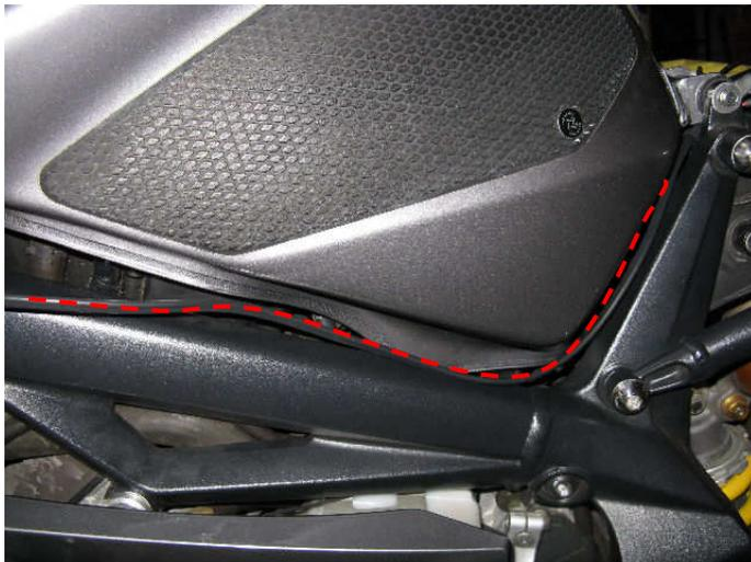
Route the wire behind the tank and frame, as indicated by the dashed line.
