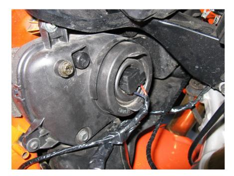
Once both headlight plugs have been done, tape up the wiring and loose terminals so they cannot short out.
