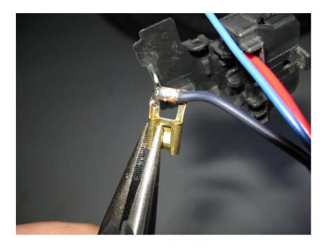
If the terminals are difficult to fit in the sockets, give the curled side a <u>very minor</u> squeeze with the pliers.
