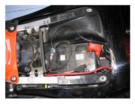
Last step, bolt the TL3 O-Ring terminals to the battery.
