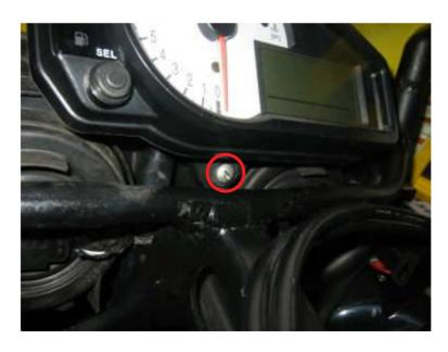
After removing the screw, the dash can be lifted out. At the back of the dash there is a rubber sheath over the wires running into it. Pull the rubber sheath back as shown in the picture below. This exposes the connector to the dash.
