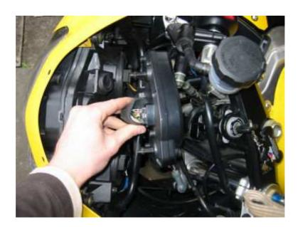
Disconnect the connector and remove the dash as shown below.
