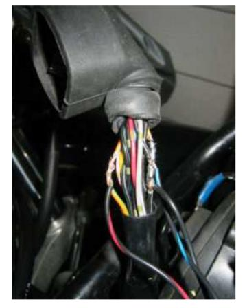
After soldering the three wires I wrapped some PVC tape around the exposed solder and copper. This is not to waterproof the connection, but to stop short circuits. This is shown in the picture below.
