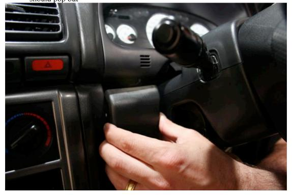
6. Remove Dash Cluster by unscrewing the 3 screws
