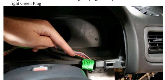
12. As per the attached wiring diagram for the WRX We only need to deal with Wire Number 9 (Orange Wire) (They are marked, some good eyes or a magnifying glass is paramount here!)
