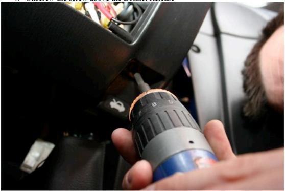
5. Pull firmly on the left hand side of the bottom part of the dashboard and it should pop out
