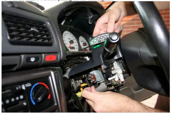
19. Put the car back together, Stick the SHIFT-I down with some double sided tape / 3M Pads.
