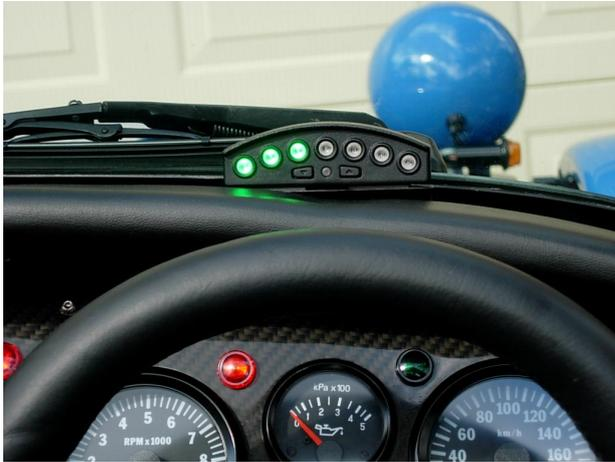
This is a great little unit, having all the functionality that could usefully be needed from a sequential shift light. It's also quite a flashy bit of kit, so if impressing your mates is important, it does that too! The nice thing about this unit is that it's fully self contained, rather having a unit for the lights and a separate control unit for the electronics and programming functions. The plastic enclosure looks neat, seems well built, and is very lightweight. It would have
