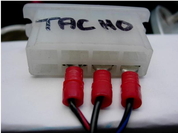
The supplied 6.4mm spades on the supplied flying leads connect Shift-I into the original tacho plug on the wiring loom.
