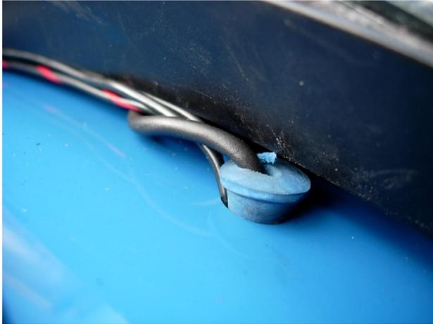
The wiring, which comes out of the top right hand corner of the unit, was routed under the base of the windscreen, and down behind the dash via an existing hole in the scuttle, normally used for the heated windscreen wire.
