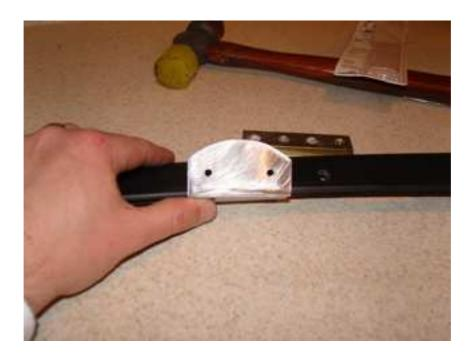
I just used a small piece of scrap aluminum (about 4"x4") and cut and fit it to the defroster vent by trial and error using a rubber mallet and a piece of steel bar (actually a seat base plate from a 964 that I had lying around).
