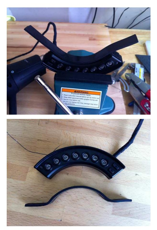
Wiring is pretty easy. The Shift-i has three wires it needs connected. Switched power (red), ground (black), and a tach signal (blue). I had seen a couple of other
