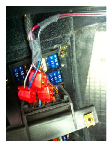
To route the wires, others had described taking apart the instrument panel and removing some of the ventilation ducting... I opted for a slightly easier approach. Took a heavy-duty 36" zip tie and fed it up from the bottom. It was pretty easy to manipulate it out the steering column opening, then I just taped the Shift-i wires to it and used it as a wire pull.
