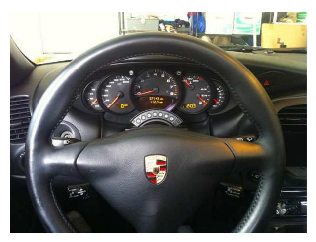
It comes in two versions, flat base or curved base. I ordered the curved base. As it turns out, the flat base might have been a bit easier to install in the spot I finally selected... No worries, I cut a small piece of Kydex and got out the heat gun to make a bracket for my curved shift light. I also used some friction tape to bundle the Shift-i wires into a harness. Closest stuff I've found to what Porsche uses for their harnesses.
