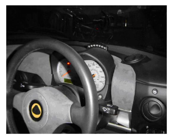
The unit is entirely programmable, and even automatically dims the LEDs depending on the ambient light. Currently I have first light coming on just after the second cam comes in, with the lights coming on at even intervals up to the final red light and flash at 8200. It all adds to that addictive second cam rush, and the mini GT racer feel of the Exige. I will probably change the settings though so the first light comes on later, say 7k ish.
