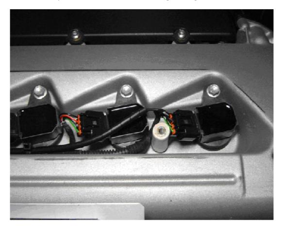
turbophil "One has to pull the signal wiring from a plug coil all the way to the dash where the light is installed." I pulled the tacho signal wire through the shifter cable access hole, up the spine and then up through a hole under the dash where the steering column goes through the bulk head. All the wires met up behind the light switches. I then fed the three very thin wires through the dash and laid them at the base of the windshield to the point where I mounted the shift light."
