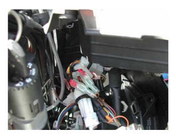
When ordering, mention to Ecliptech you have a KTM950, so they can crimp spade terminals on the Shift-I wires for you. Then they conveniently plug in.
