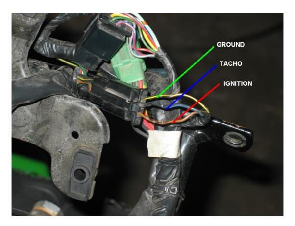
You can either solder the wires or use the wire clips that come with the Shift-I.
