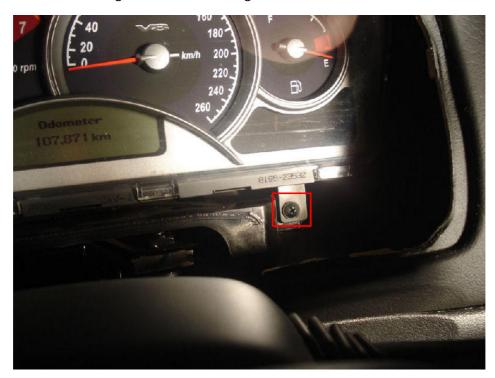
4. Remove mounting screw at the bottom right. To access this a little easier I removed the sensor in front of the screw
