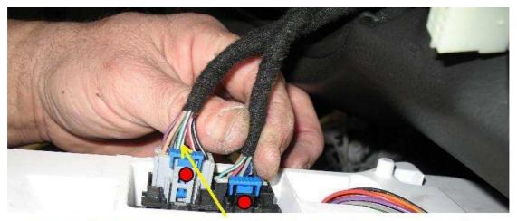
Arrow points to "white" wire that you can tap into for RPM signal on C6 Corvette This is the connector on the rear of the instrument cluster
