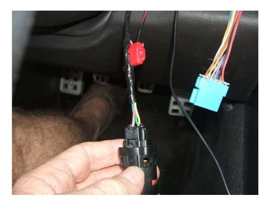
For an RPM signal I tapped into the white wire in the connector that goes to the Tacho on the back of the instrument cluster.
