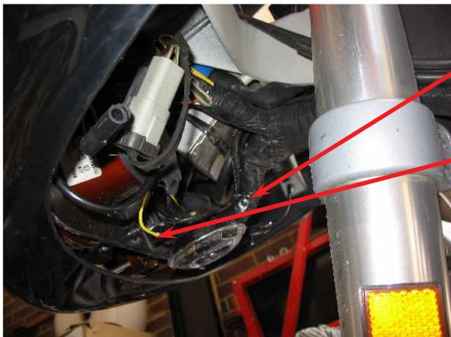
The wires we want to get to are here. Take the cable ties off.
