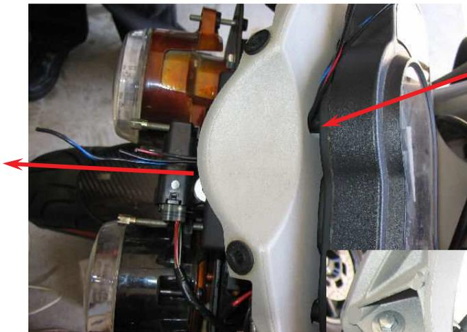
Thread the Shift-I wires through holes behind the instrument.
