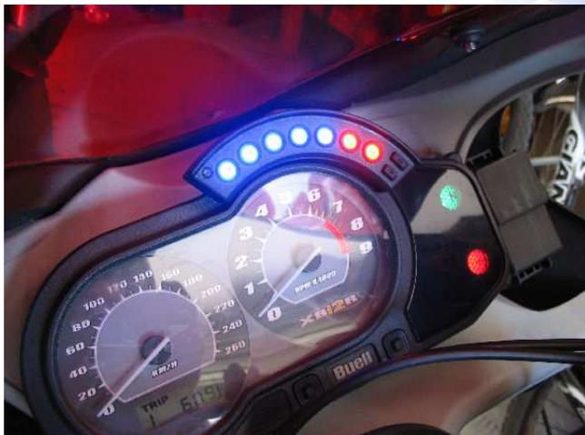
The Shift-I has a calibration setting that you need to change. This setting is just to match the Shift-I to the Buell's tacho signal. Hold both buttons down, turn ignition on and let them go. You will have 2 lights showing (calibration default is 2). Press down twice, now 1 light showing (calibration 1). Press both buttons together to save the setting.
