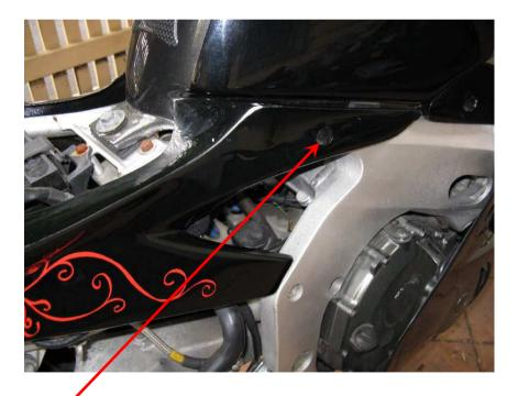
After the bolts below are removed, you can remove the rear tail fairing.
