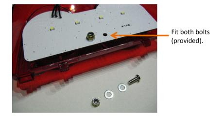
When re-assembling the lens to the white bracket, it's a good idea to soak the <u>white bracket</u> in hot water again to soften the glue. **But DO NOT put the lens with the LED module into the water!**
