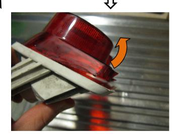
Lift bottom edge up to the position as shown.
