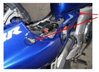
Remove the 4 fairing bolts, using a 5mm Allen key.
