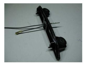
With all 3 wires passed through the backplate, fit the clear rubber jackets to the female bullet terminals, as shown below.
