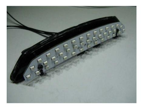
Use a silicone to bond the lens to the back plate. Preference is for an automotive silicon commonly found at automotive stores. Sikaflex 227. A small tube is ~\$16.
