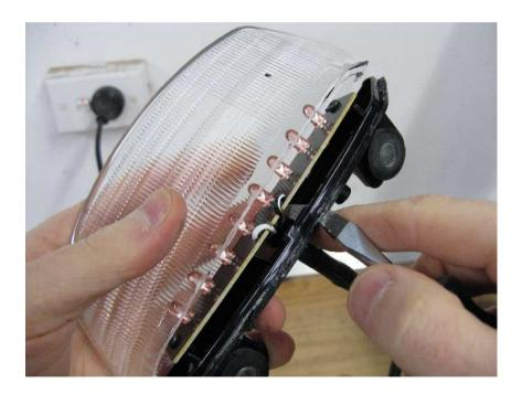
Remove the two screws holding the LED panel on. Cut the wires and remove the wiring from the backplate. Feed the wires from the new upgrade module through the hole in the backplate. One at a time, starting with ones with the extra terminals.
