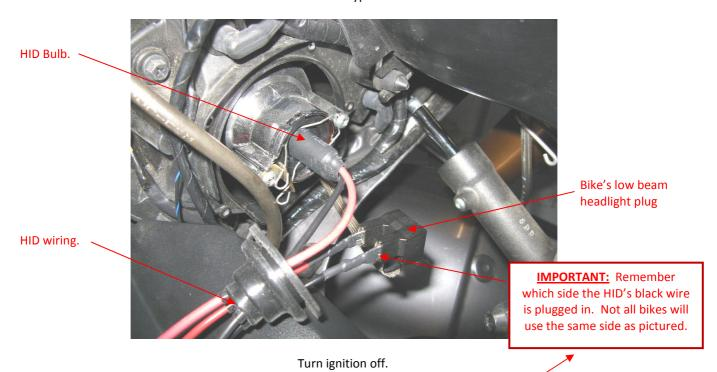
Before unplugging in the HID, take note of where it's black wire is plugged into the headlight socket.
